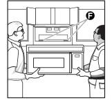
mounting plate. Set the microwave oven aside on a protected surface.
